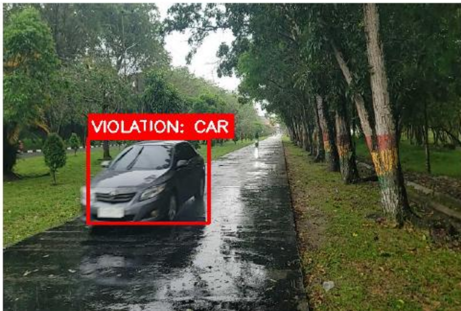
Figure 3. Speed Violation Detection Results under Light Rain Conditions
