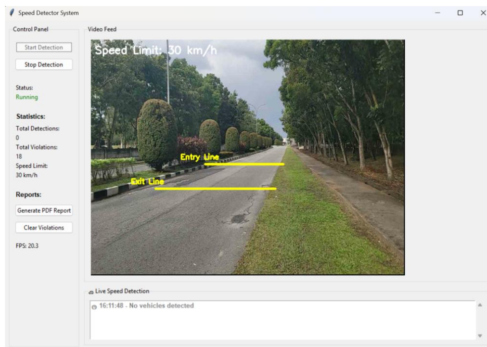
Figure 2. A two-line virtual measurement approach
