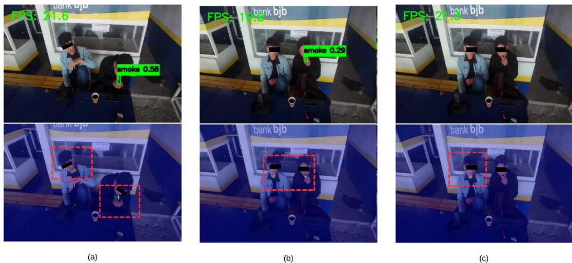
Figure 3. ADAM's performance in limited-object smoking activity detection scenario: (a) initial detection of smoking activity with adaptive heatmap generation in the region of interest (highlighted in red box), (b) transition phase showing
