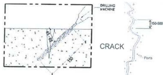
Gambar 7 Drilling Crack Area
